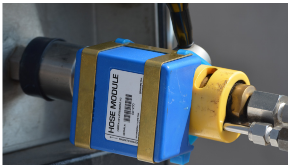
Hose Module on CNG pump.
